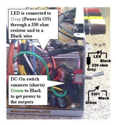
Check for loose connections by gently tugging on them. Inspect for bare wire, and cover it to prevent a short circuit. Put a drop of super-glue to stick the LED to its hole. Put the cover back on.
