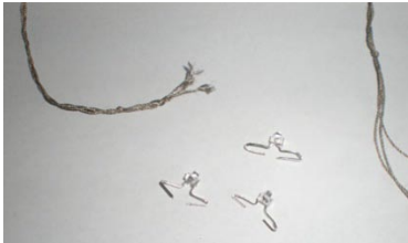
Plate 1: Twisted Conductive Threads and Modified LEDs
