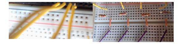
Next you want to connect four wires top ins 2 till 5, the other side of the wires are connected on the breadboard 2 holes away from the resistor. You can choose to put these further away but I didn't have much space to work with.
