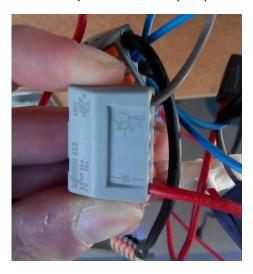
The last step for the pump wiring is to connect the positive wire from your plug to 4 different wires this will be needed for the relay board.
