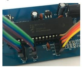
Connect the pins from the Board as bellow, The colours of the ribbon cables may vary.
