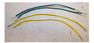
Remove 5 to 7mm of insulation off both ends of the 4 stranded wires
