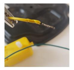
Apply solder to the other end of the wires (tinning) to create a solid section of exposed wire (this will make it easier to connect to the motor controller) 4
