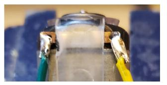
Solder the stranded wires to the geared robot motors so the wires are hanging down past the robot motor shaft. Put one of each color on each motor (use the same color side alignment on each motor - ex: yellow wire on the left)
