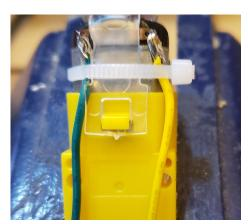
Tighten a zip tie around the motor housing over the wires (This prevents the copper tab on the motor from breaking)
