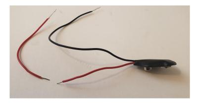
Expose 10 mm of wire the 9v battery snap wires (only 3 or 4 will be showing)
