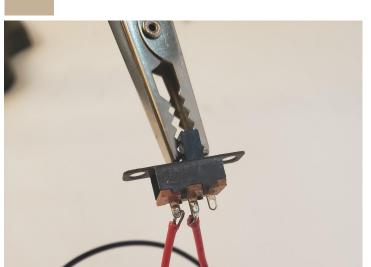
Solder both red wires to the ON/OFF switch terminals as shown.
