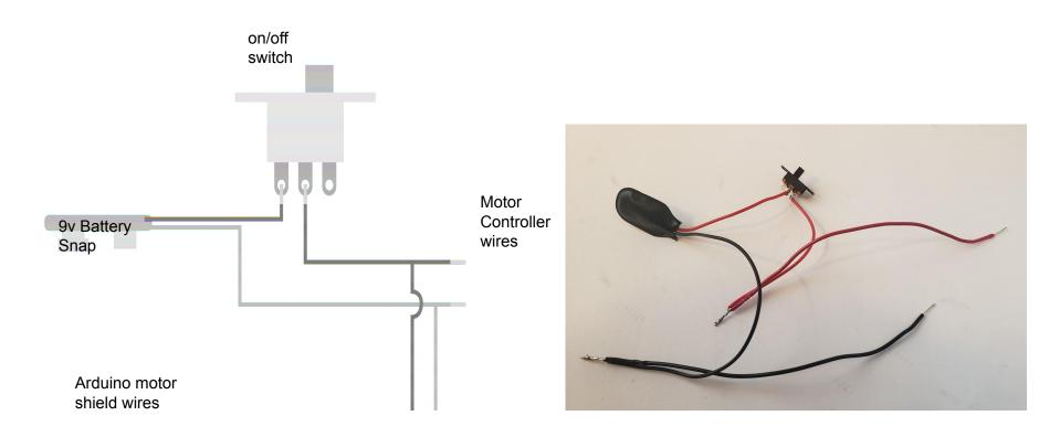
Examine the Power Wiring Harness Diagram. This shows the electrical connections necessary to provide battery power to tBB
