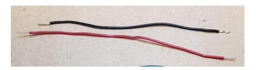
Expose 5 to 7mm of wire on red and black solid core wires
