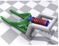
With a mono-shock rear suspension, a single shock absorber connects the rear swing arm to the motorcycle's frame. Typically this lone shock absorber is in front of the rear wheel, and uses a linkage to connect to the swing arm. Such linkages are frequently designed to give a rising rate of damping for the rear. Mono-shocks are said to eliminate torque to the swing arm and provide more consistent handling and braking.
