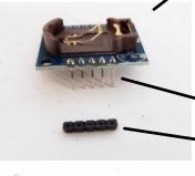
IF YOU ARE USING HOLDERS FOR NANO AND CLOCK CUT THE STRIP AND NOTE PINS 3-13-14 HAVE BEEN REMOVED
