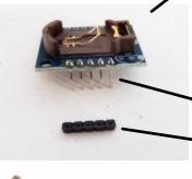
IF YOU ARE USING HOLDERS FOR NANO AND CLOCK CUT THE STRIP AND NOTE PINS 3-13-14 HAVE BEEN REMOVED
