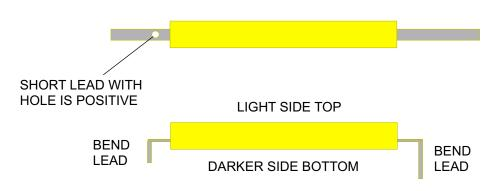
USING HOLDER FIT TWO FILAMENTS IN - BE CAREFUL, DON'T FORCE IN. THE FILAMENT IS EASILY BROKEN
