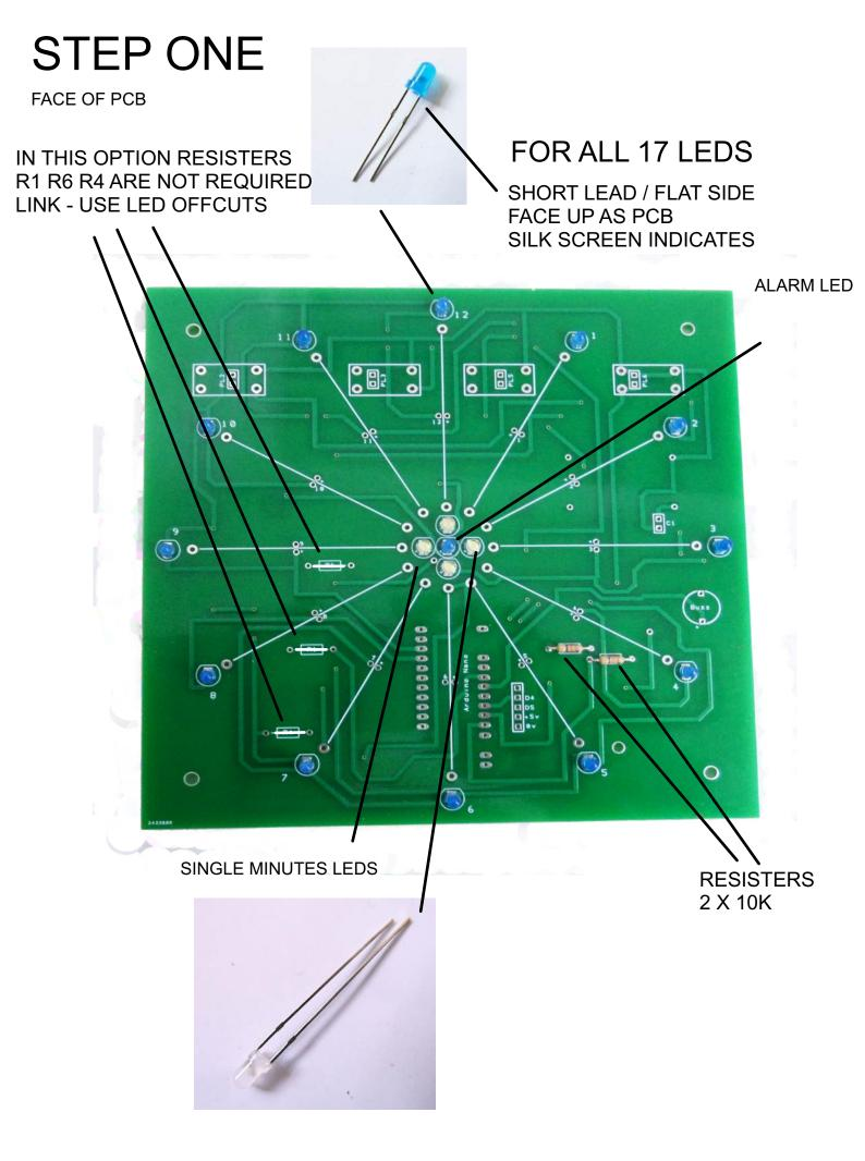
NOTE - DON'T DISCARD THE LED LEADS AFTER CUTTING NEEDED IN STEP 2
