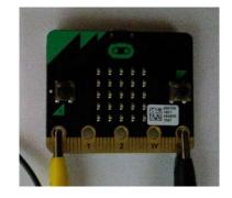
Connect one end of one crocodile clip to the **pin labelled 0**.
