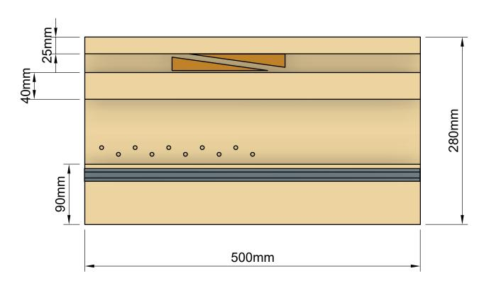
Except for the wedges, all parts from 19mm (3/4") plywood
