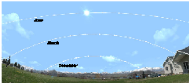
FIG. 1: Different solar tracks across the sky as a function of the time of year, as viewed by a northern hemisphere observer standing facing south.
