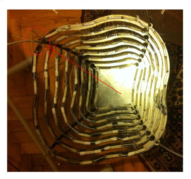
As you see above, all the power wires, from bottom to top are connected in sequence to each other to provide energy to all the LEDs. And the main wire at the top is connected to the power adapter.
