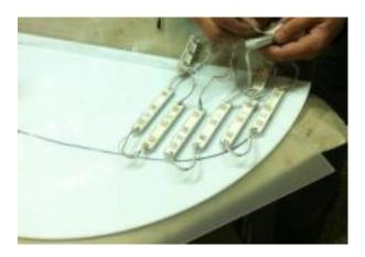
I sticked all the LEDs on the plexiglass. After sticking process, I obtained steel wire, clamps, smooth and surface aluminium pipe to assemble all parts of my desgin .
