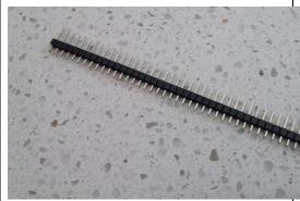
Straight header pins – for plugging the shield into the Arduino Uno.
