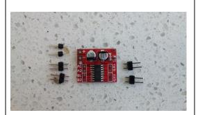
Use header pins to mount the break-out board onto the shield. Solder the header pins to the break-out board and on the shield. Cut off excess length of the header pins.
