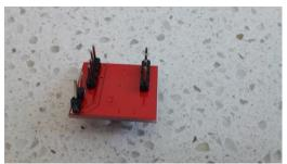
The robot shield PCB has been designed for the breakout board which has a 3mm spacing between the Motor A and Motor B pin sets, and between A and B input pin sets. However, it is possible you will get the break-out board with closer spacing's at 2.5mm.
