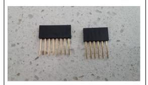
6 pin and 8 pin female long needle header strip, e.g.
