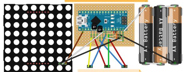
The 2-pin headers here represent the banana plugs to connect the banana jack colors and cube faces faces together.
