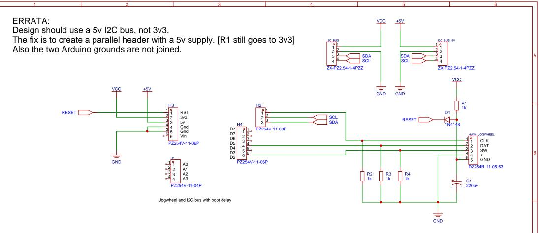
Used NodeMCU Amica2 as the base footprint, emulated it with headers then deleted it off the board, else you create two board headers
