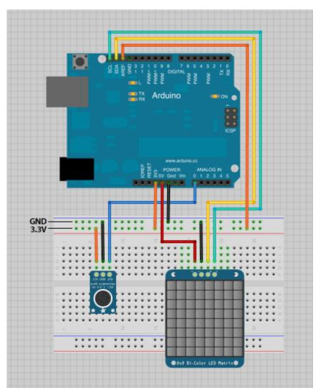
If using a "classic" Arduino board — an Arduino Uno version R1 or R2, Arduino Duemilanove or Diecimila (with 328P chip), the matrix data and clock lines should be connected to analog pins 4 and 5:
