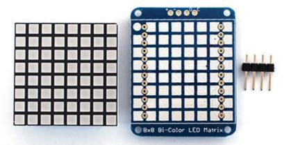
If working with a breadboard as we show below, solder row headers on to the microphone breakout and LED matrix backpack boards (three pins on the former, four on the latter). You can optionally use 90 degree headers if you'd like either component to be positioned standing up. Thanks to the "smarts" of the LED matrix backpack, this whole project requires fewer than a dozen connections total:
