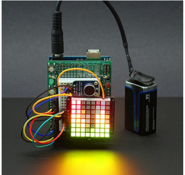
Depending how you choose to orient the LED matrix, the matrix.setRotation() function can be used to keep the graph upright.
