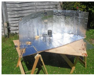
Cardboard baseplate 48x18 inches. I used 3ply board to make it reasonably rigid. It can fold in half for transport forming an 18x24" briefcase format. Handholds are cut in each half.
