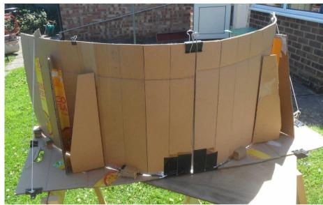
The parabola is supported in use by some buttresses; these are glued to the back of it and can fold flat for transport. Two tensioning strings are tied to clips on the base. They have a square of cardboard tied to one end; the string slips through a small slot at the joint between two These pull against the buttresses to keep them in place on the base. It is further aligned by small cardboard blocks glued to the base; these will marginally reduce efficiency by creating a
