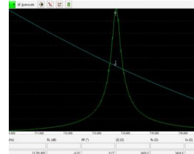
This is the adjusted antenna tuning at  $f_{res}=13.8\text{MHz}$
