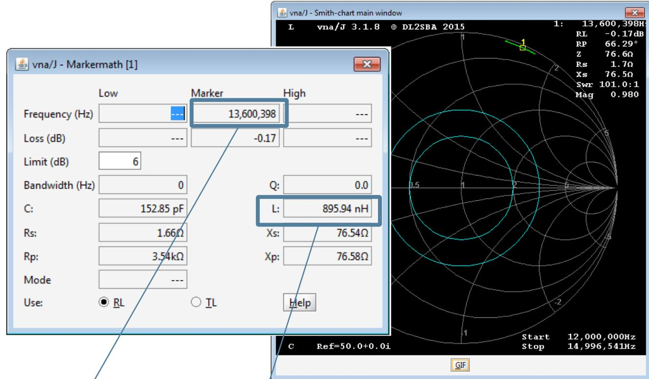
$$f_{\text{res}} \sim 13.6 \text{ MHz} \quad L_a \sim 895 \text{ nH}$$
