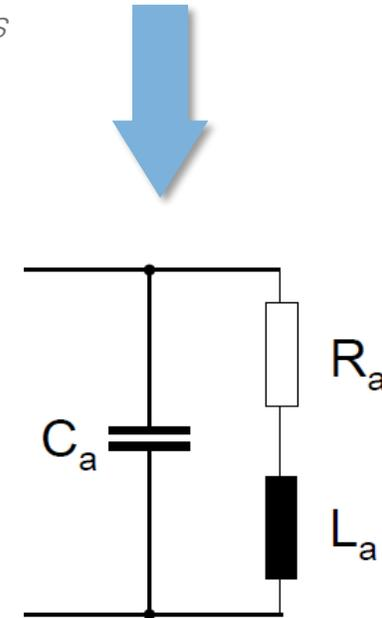
Fig. Antenna series equivalent circuit
