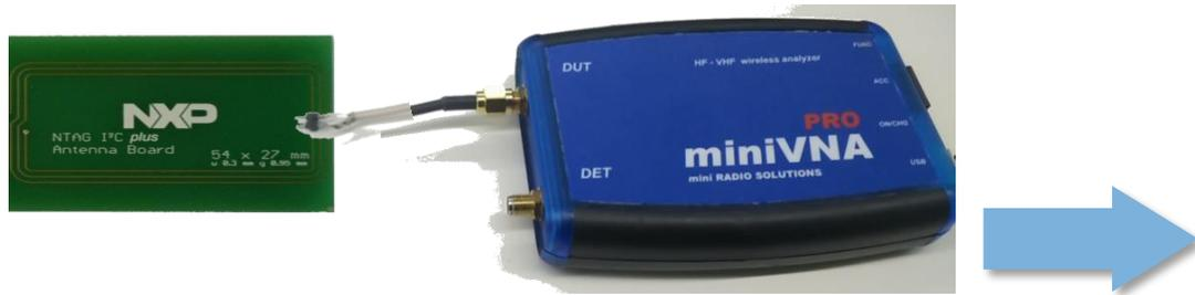
Fig 1. miniVNA PRO network analyzer connected to the 54x27mm PCB antenna connectors
