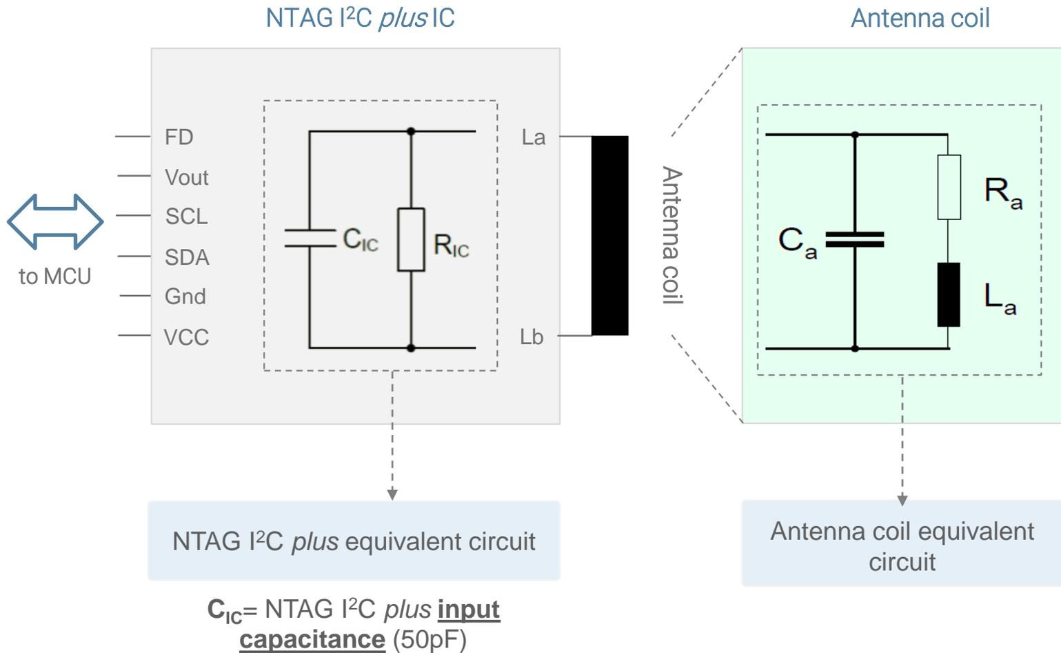
Each antenna is a resonant circuit with a specific input impedance.
