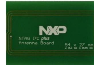
We separate the NTAG I<sup>2</sup>C *plus* from the PCB board to characterize the antenna parameters
