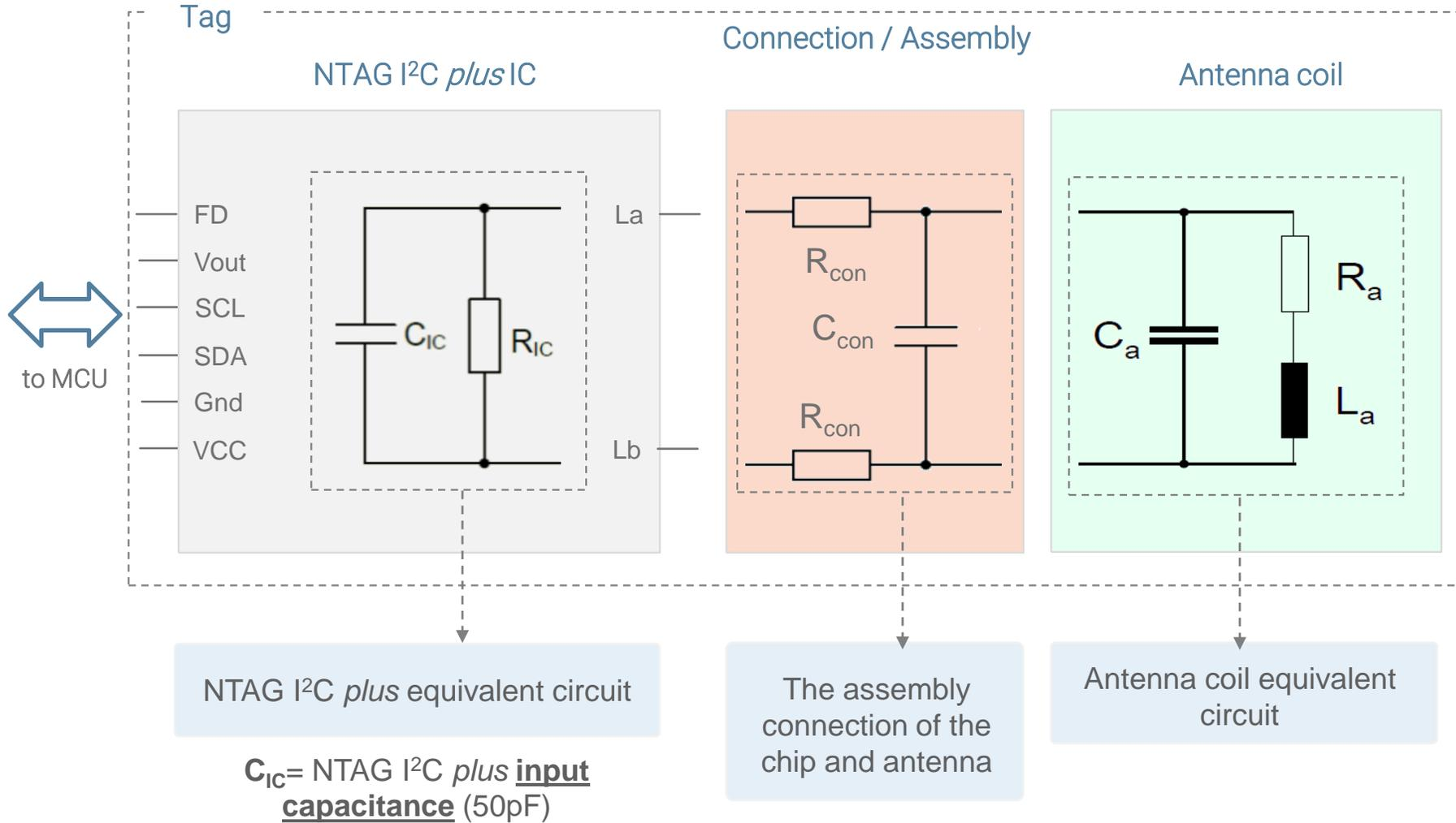
The NTAG I<sup>2</sup>C *plus* capacitance together with the antenna capacitance and the parasitic connection capacitance forms a resonance circuit with the inductance of the antenna.
