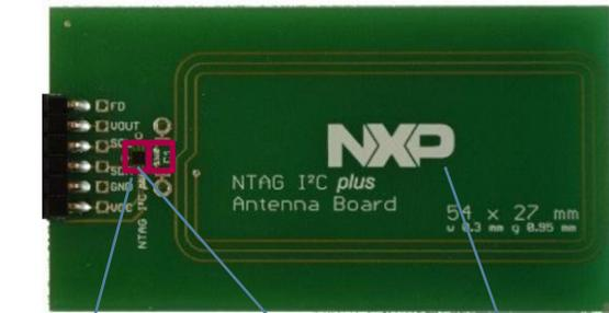
NTAG I2C plus IC       $C_{Res}$  (100pf)      Antenna coil
