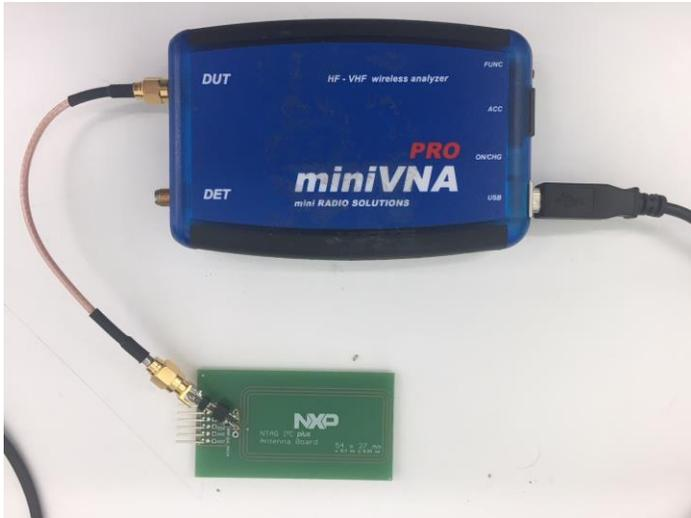
Fig 1. 54x27mm PCB antenna + NTAG I<sup>2</sup>C plus connected to miniVNA PRO
