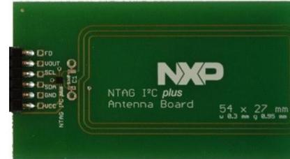
We selected 54x27mm PCB antenna board included in [OM5569-NT322E](#) kit
