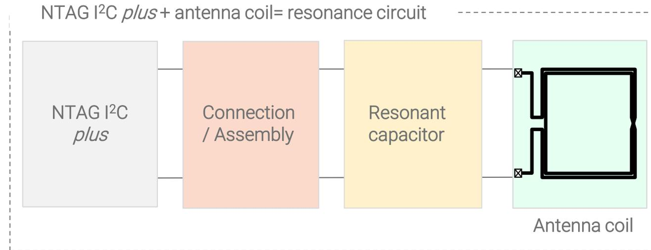
The precision of the antenna equivalent inductance computation, the length of the connection between the chip and its antenna, and the environment (metal surface, ferromagnetic material) impact the tuning frequency.
