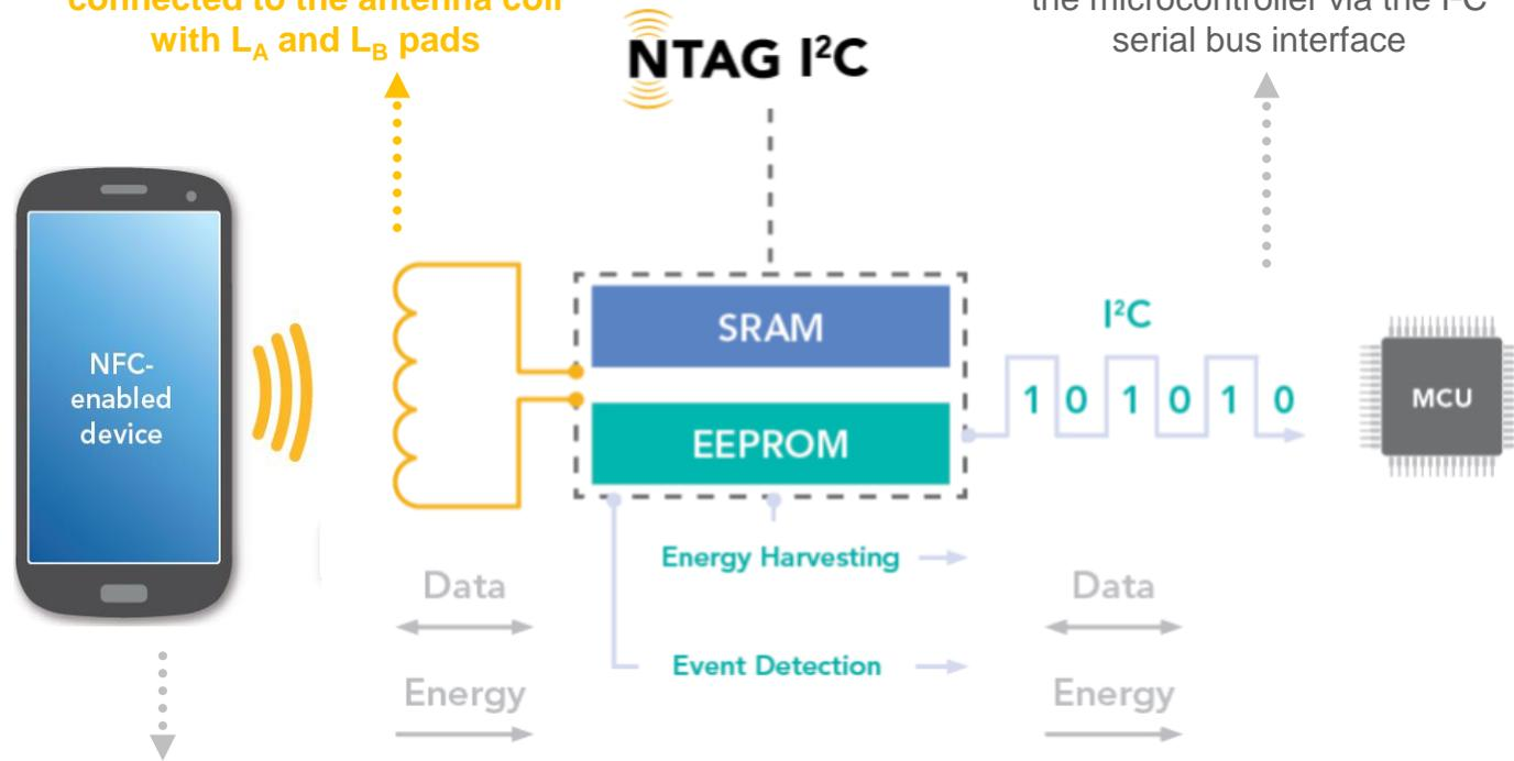
The NTAG I<sup>2</sup>C *plus* connects to the microcontroller via the I<sup>2</sup>C serial bus interface
