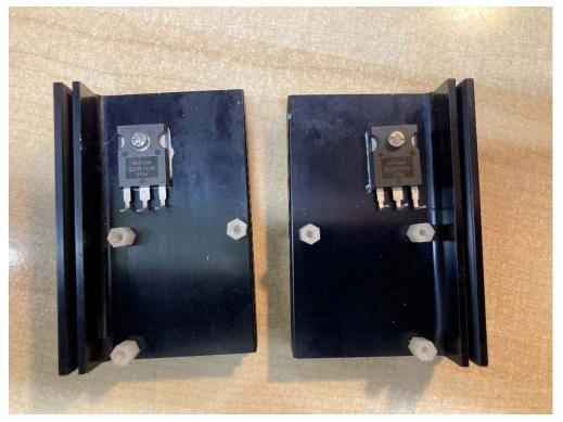
Next, I place the PCb on top and solder the pins of the mosfets. Take not how I used isolated spacers! Also, make sure that the heatsinks don't touch! The left and right channel have to stay separated. If you are using 1 heatsink and not two, you will have to isolate the mosfet from the heatsink using thermal pads.
