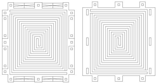
6. You have to add on the joints to hold the sides together as shown above. The spirals are the same just turned 90 degrees.
