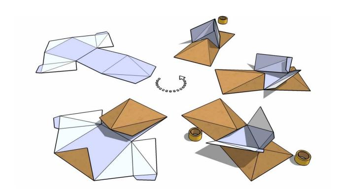
${ ext{--}5.4}$ : start folding cardboard part c, and tape where you see the tape symbol (follow the arrow in the middle for each folding step)
