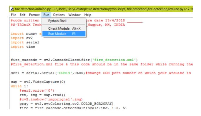
If all connections are ok, camera preview will show on screen. Now show fire to it, fire get detected and pump start as well as buzzer starts beep sound.
