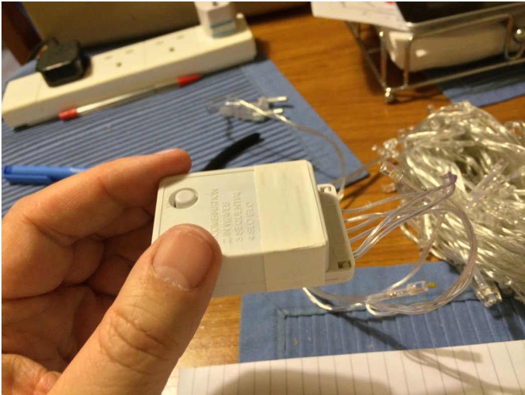
Front of control box after completion. LED's will no longer FLASH
