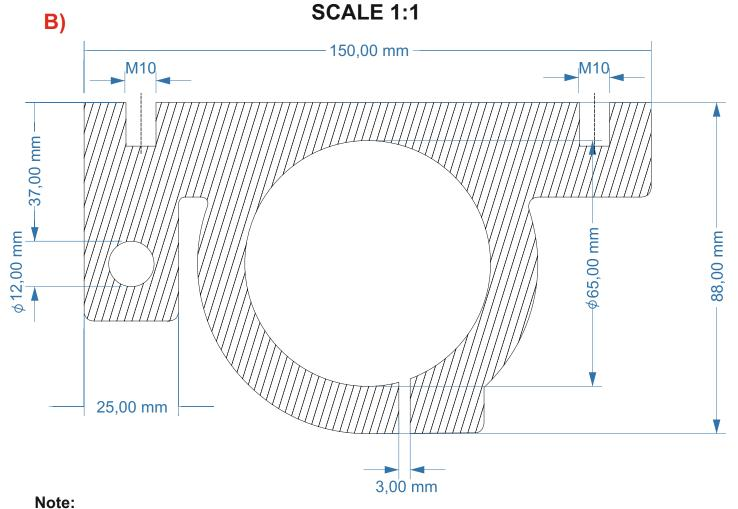
material thickness: 15mm M5 (metric thread) / drill hole 4mm M10 (metric thread)/ drill hole 8mm
