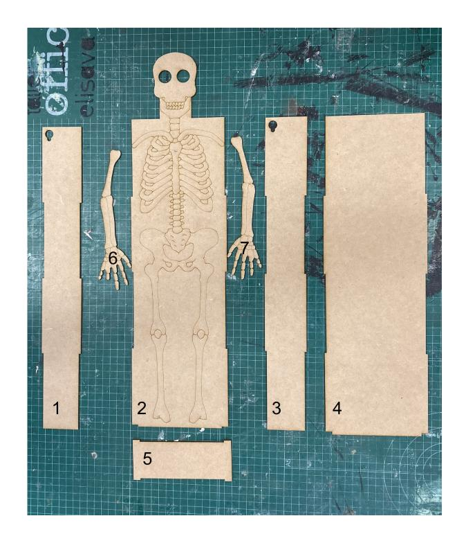
Once you have all the pieces cut you can join them by using white glue. You should glue all parts except **2** and **both arms**, it is important to keep the structure open in order to install the circuit. Once the laterals and the back part are joined with glue you can make the union stronger with a silicon gun.
