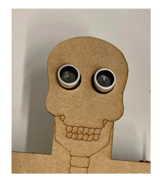
Before connecting the components to the protoboard, you should attach the servos to the holes of parts 1 and 3 and the ultrasonic sensor to the eye's holes. When you have the electric circuit ready, following the protoboard scheme, you can attach the arms to the servos.
