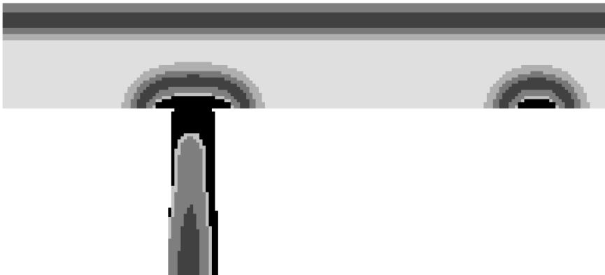
Fig. 2. Predictions of chloride concentrations development for 30 years – detail around the supporting pier with critical concentration region (black)
