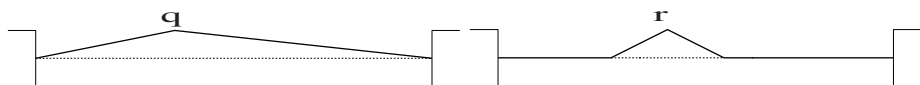
Fig. 3. Initial states of plucked string and struck string. Dashed lines represent state of a string in equilibrium, and thick solid lines represent initial state of plucked string or struck string. q is the plucking position and r is striking position.
