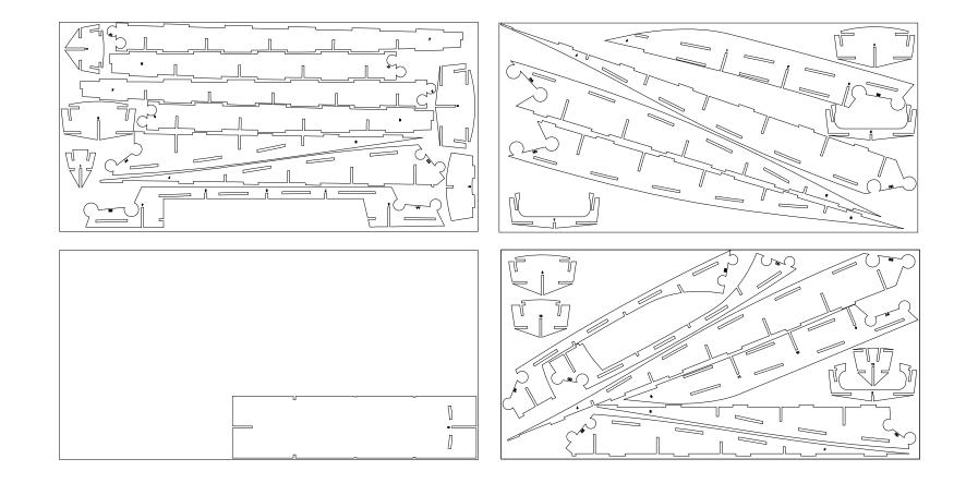
Parts to be cut from 4 sheets of 1/2"x4'x8' Hexacomb Cardboard Red lines to be cut through. Blue lines to be a light etch.
