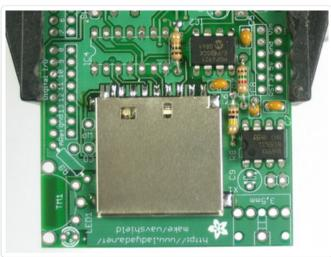
Next is the operational-amplifier (op-amp) **IC3**. It is used to buffer and amplify the output, so that it can drive a small speaker or headphones.
