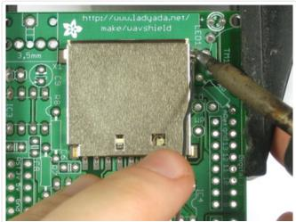
soldering iron, then poke just a bit of solder in.
