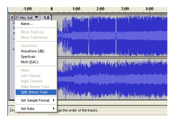
Next, when you mix a track you'll end up adding both of them together. This means that if both sides are loud, you'll get distortion. Reduce the gain on both tracks to -6dB.
