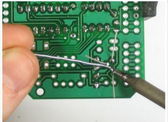
Turn the board over and solder/clip the three leads.
