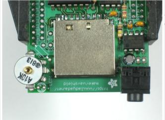
Next is the volume potentiometer **TM1**. This is an audio-type 10K pot. It will slip into place pretty easily.
