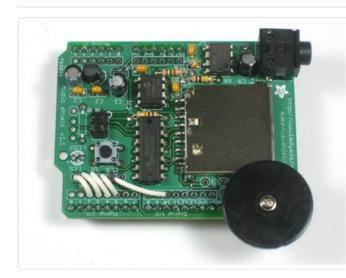
Pins 13, 12 and 11 are used to talk to the SD card and cant be changed. The rest of the pins, however, are more flexible. Still, for all the examples on the site we'll be using this wiring, so it is suggested to just go with this.
