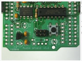
Next is the reset button and the ICSP header. These let you reset the Arduino manually, and reprogram it directly with a AVR programmer.
