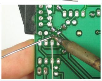
Solder and clip the small capacitor leads.
