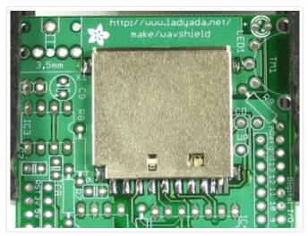
Next, we will solder all of the many resistors. The 10K resistor **R6** is first.
