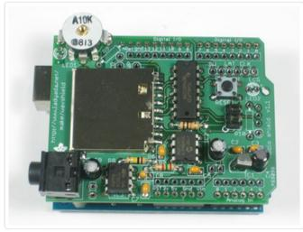
Place the shield PCB onto the arduino so that all the holes match up with the header.
