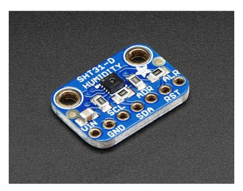
Sensirion Temperature/Humidity sensors are some of the finest & highest-accuracy devices you can get. And, *finally* we have some that have a true I2C interface for easy reading. The **SHT31-D** sensor has an excellent  $\pm 2\%$  relative humidity and  $\pm 0.3^{\circ}$ C accuracy for most uses.
