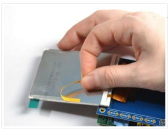
Now we can attach the screen. Remove the two thin tape cover strips.
