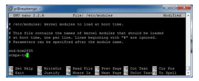
Save the file and reboot the Pi with **sudo reboot** and look at the console output (or run **dmesg** in the console window after logging in) you will see the modules install. Look in particular for the STMPE610 detection and the ILI9340 screen frequency as highlighted here
