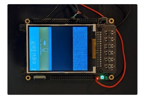
Because there are several incompatible versions of the Kaluga TFT display, the bootloader's screen may appear incorrectly or not at all. This does not affect its operation.
