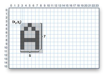
Text is very flexible but operates a bit differently. Instead of one procedure, the text size, color and position are set up in separate functions and then the print() function is used — this makes it easy and provides all of the same string and number formatting capabilities of the familiar Serial.print() function!
