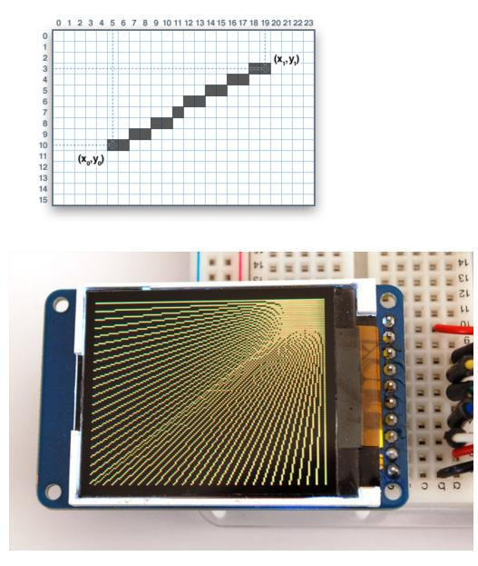
For horizontal or vertical lines, there are optimized line-drawing functions that avoid the angular calculations:
