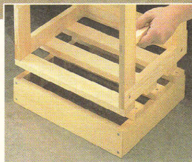
▲ The interlocking design of these crates allows you to stack them in different configurations and move them around easily.
