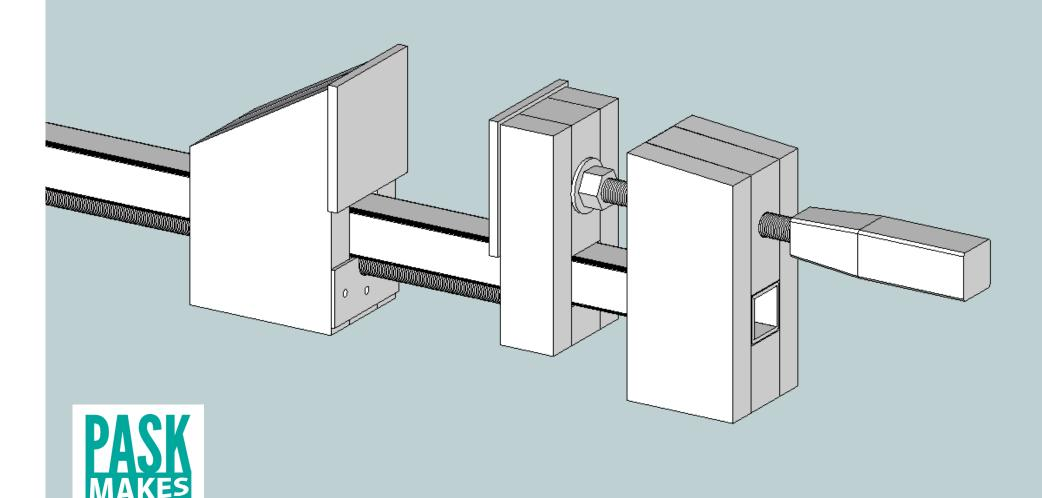
These clamps are an easier to make version of steel clamps I made a while ago - unfortunately I didn't make plans for those clamps but these plans could be of help if you wanted to make the steel ones. These clamps, while not being quite as heavy duty as the steel clamps, still have plenty of clamping pressure for any glue up and they should still last for years.
