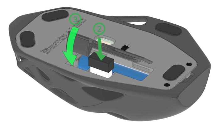
② Insert the 2.4G module. ③ Press down and snap on the battery cover.
