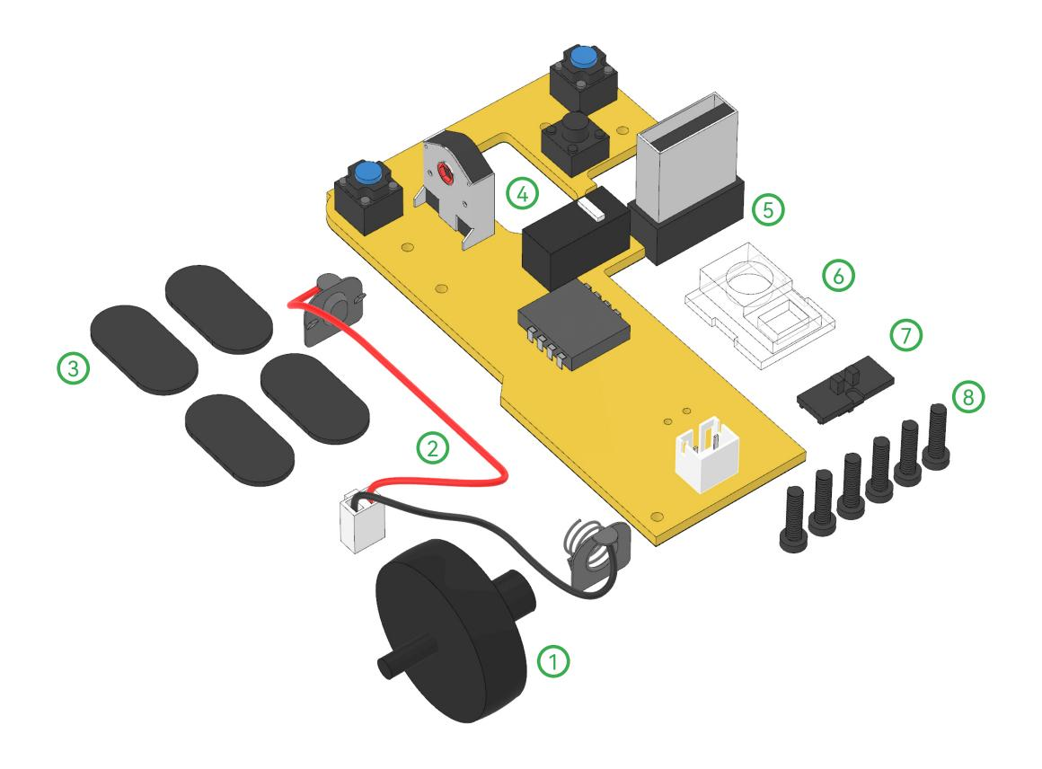
① Scroll Wheel ② Power wires ③ Mouse Foot Pads (x4) ④ PCB Board ⑤ 2.4G Module ⑥ Lens
