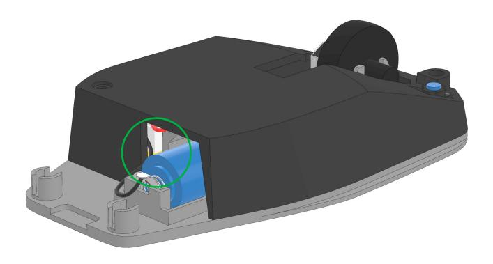
① Be careful to avoid pressure on the wires from the PCB cover plate.
