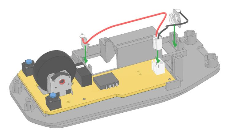
① Insert the positive and negative terminals, as well as the socket, into their respective slots.
