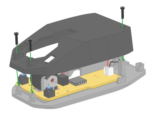
② Secure the PCB cover plate to the base plate using 3 screws.
