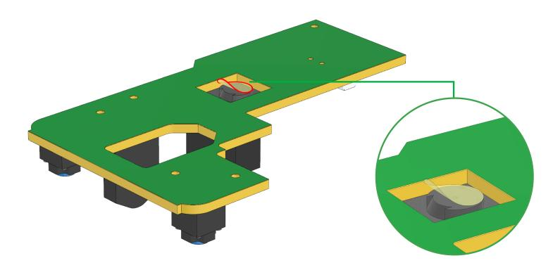
① Remove the protective film from the sensor surface.
