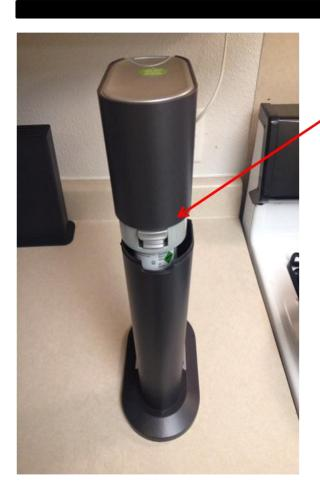
If done correctly, the top half should separate from the bottom half which will expose the Co2 bottle .
