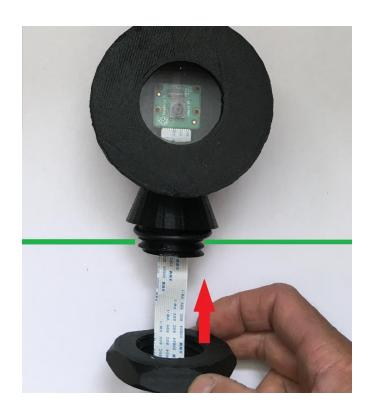
9. Connect the free end of the ribbon cable onto your other equipment (ex: Raspberry Pi computer board) and test it out. If the Raspberry Pi camera board is not suitably level within the WeatherBox, the rim of the WeatherBox might be visible in your pictures. Unscrew and remove the plexiglass plate and O-ring, and use the erasure from a pencil or similar device to genly poke down the corners of the circuit board.
