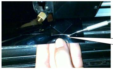
Test pattern cut completely through the backing paper using 80grams of cut force.
