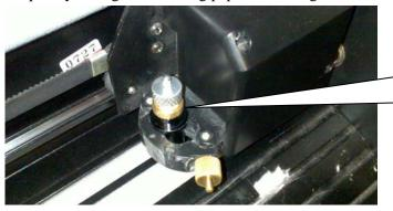
MH1351 shown with cutting tool properly installed in the upper portion of the tool holder clamp.
