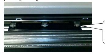
MH1351 shown holding a 12-inch wide vinyl sheet with 3 feed wheels spaced evenly across the sheet.
