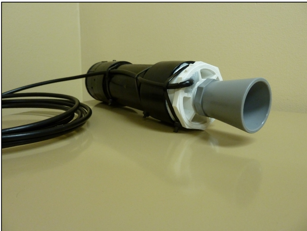
Figure 6: External antenna cable inserted through case bottom and sealed with silicon.
