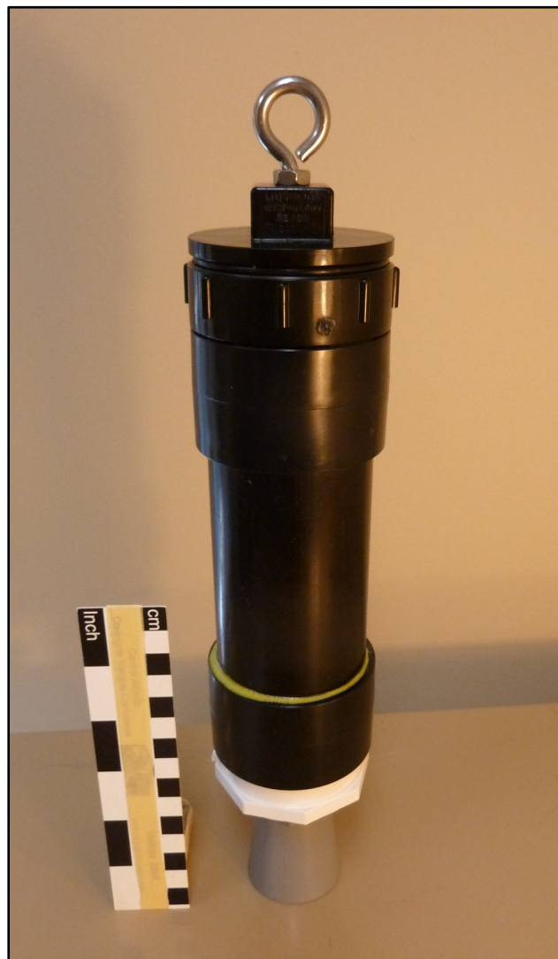
Figure 1: External view of meter. Dimensions: 320 mm long (tip to tip), 50 mm diameter.
