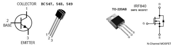
BC547 PNP transistor and IRF840 MOSFET pinouts
