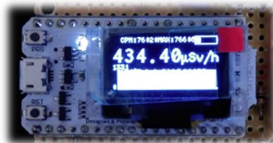
Saturation during the tests with a radioactive source
