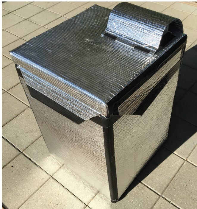
The fully assembled cooler, sealed and protected from direct sunlight by silver bubble wrap insulation.
