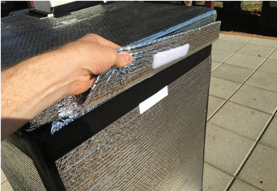
Top of cooler box is secured by hook and loop fasteners on each of four flaps.
