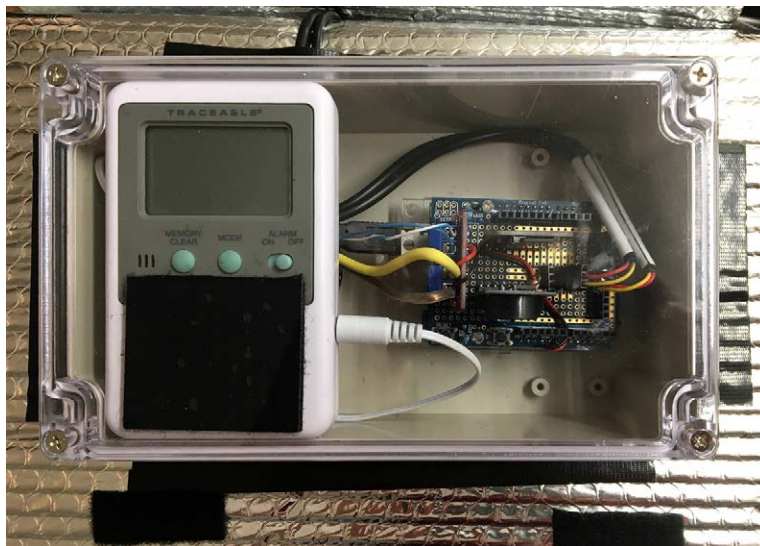
The electronics box contains a calibrated vaccine thermometer (left) and the Arduino UNO with custom shield (right). All wires feed down through bottom of box and through the cooler's lid.
