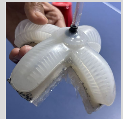
3D printed soft gripper with cloth base
