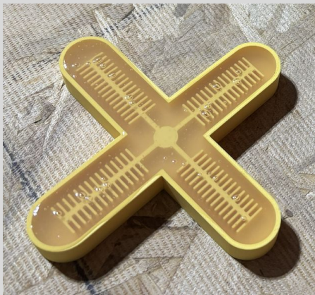
Quadrupedal Soft Gripper with central air chamber using 3D printed mold
