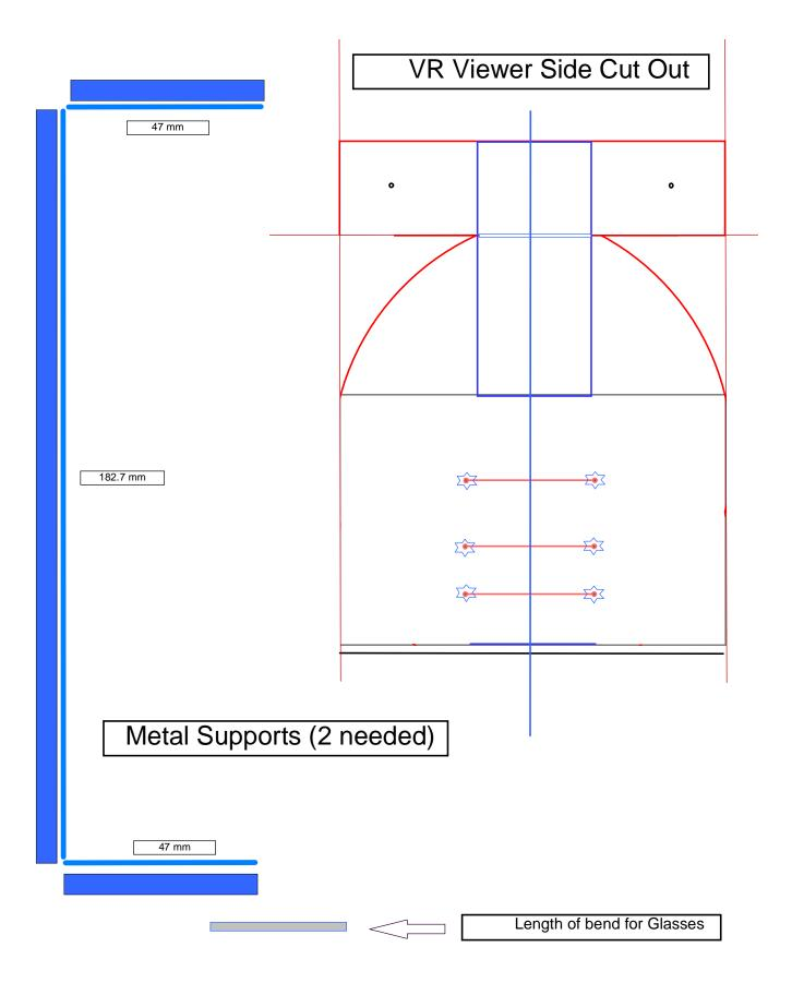
Black means score. Red means score and cut. Blue means informational. Star means drill use 1/8 bit.
