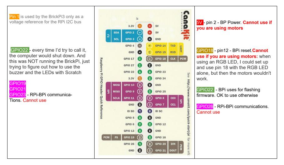
This information is from the DexterIndustries.com BrickPi forums: Can you use the BrickPi GPIO pins, correct as of July 2018.
