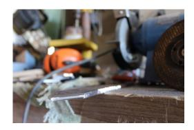
DO THE THINNING ON THE SIDE OF THE BLADE THAT IS GOING TO STAY CLOSE TO THE HANDLE TO MAKE A PLACE FOR YOUR FINGER.
