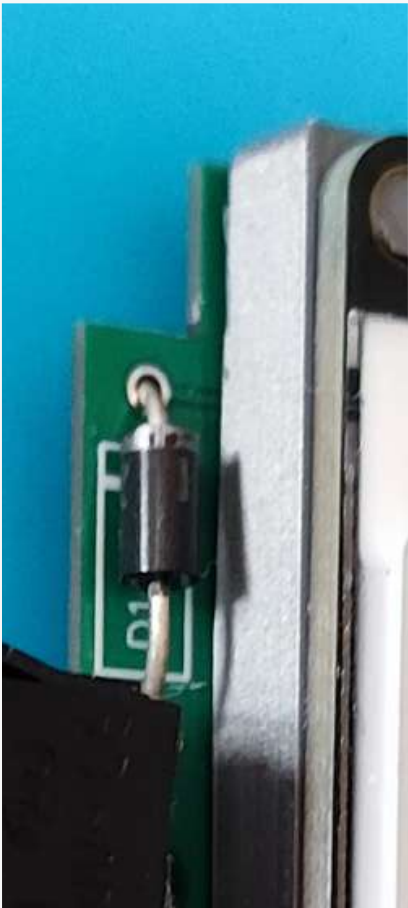
The gray line of the diode must be upwards (opposite the Power button)
