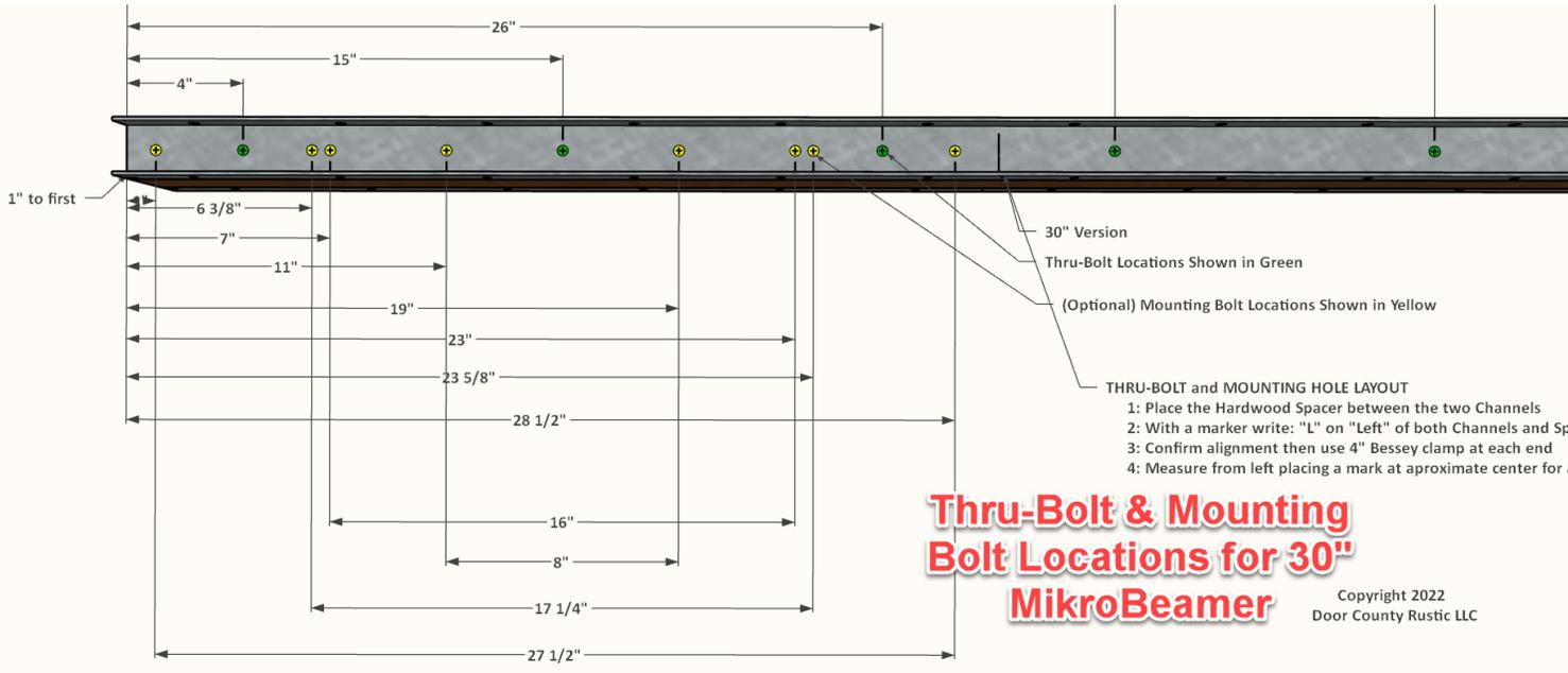
**Thru-Bolt & Mounting Bolt Locations for 30" MikroBeamer**
