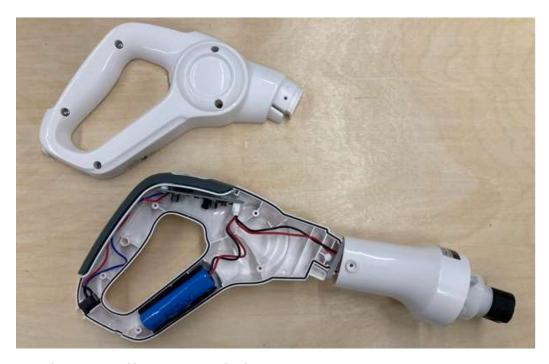
8. Carefully pull off the top half of the handle to expose the electronics.
