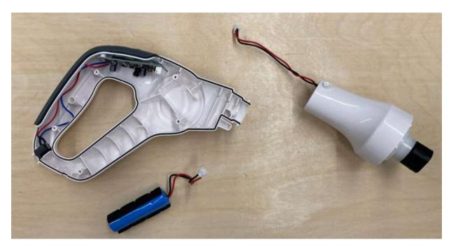
10. Remove the battery and detach the scrubber end.
