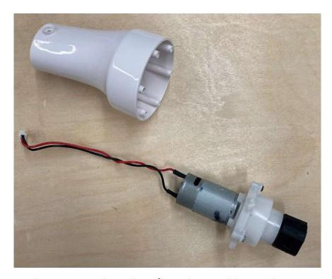
11. Slide out the motor and gearbox from the scrubber end.
