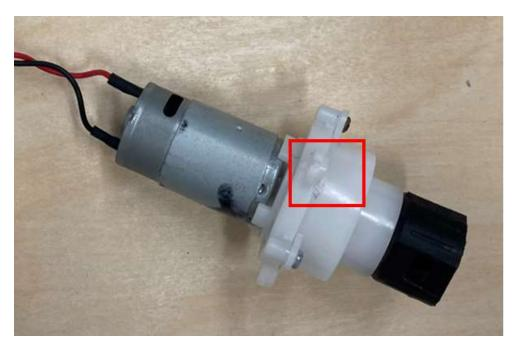
12. Use a Dremel Cutting Tool or Horizontal Bandsaw to remove the hollow cylindrical extrusions that held the Gearbox Screws. Cut so that only flat tabs with screw holes remain. This will allow the gearbox to be installed properly in future steps.
