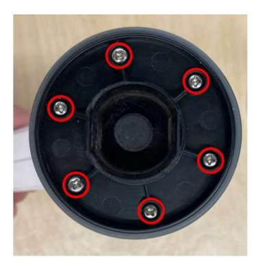
Use a screwdriver to remove the 6 screws that connect the round black motor cover at the scrubber end. Set these screws aside because they will be used during assembly. They will be referred to as the **Motor End** Screws.
