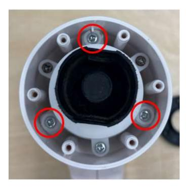
4. Use a screwdriver to remove the three screws connecting the gearbox to the scrubber. These can be identified with the wide tabs. Set these screws aside because they will be used during assembly. They will be referred to as the **Gearbox Screws**. Do not remove the other three screws because they hold the gearbox together.
