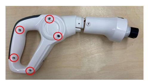
7. Use a screwdriver to remove the 5 screws that hold together the two halves of the handle.
