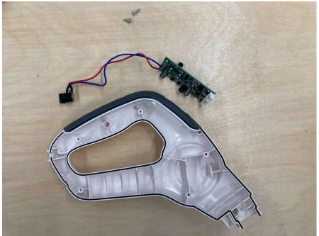
13. Use a screwdriver to remove the two screws mounting the PCB to the bottom half of the handle. Set these two screws aside because they will be used during assembly. They will be referred to as the **PCB Mounting**Screws. Carefully remove the PCB and Power Jack from the handle.
